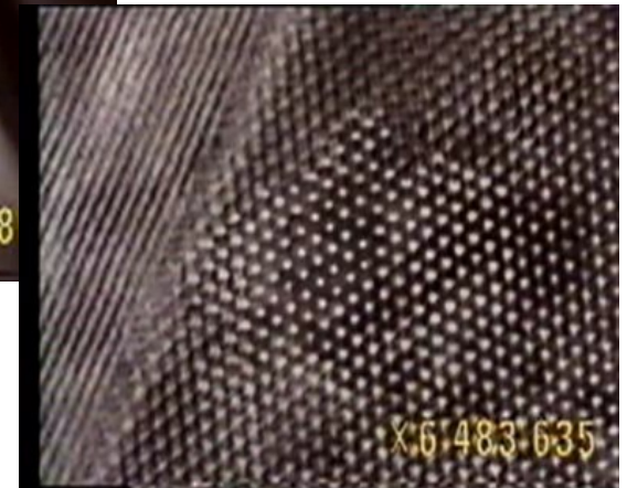
Structure atomique \text{Al}_2\text{O}_3 (0.1 nm)
